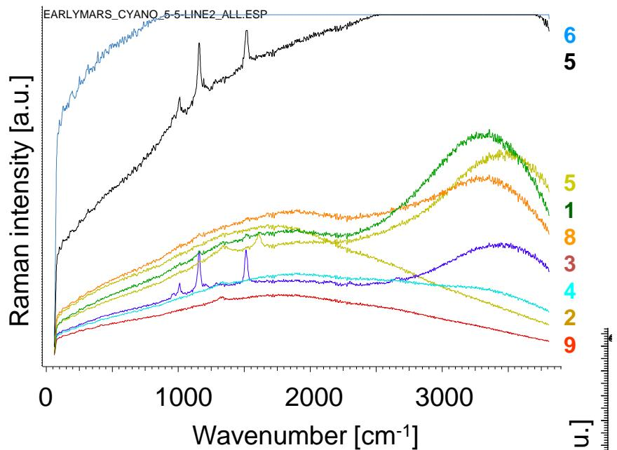
Typical Raman spectra of the line scan (20s, 5x).
